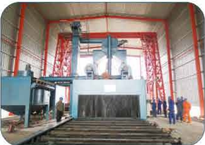
抛丸除锈 Shot blasting
